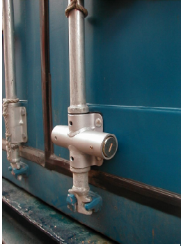
CC Bearing Bracket 1 Fabriksmonteret.
